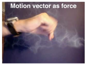
Example 8. Motion vectors and normal maps are combined and used as a constant vector force to affect the particles after birth. As the object moves through the frame, the force from the vectors pushes the particles out of the way along the vector of motion, and away from the surface.
